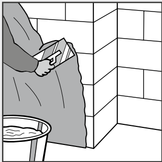
Figure 18: On chimney walls a layer of bonding compound is applied and the fermacell boards floated into position.
