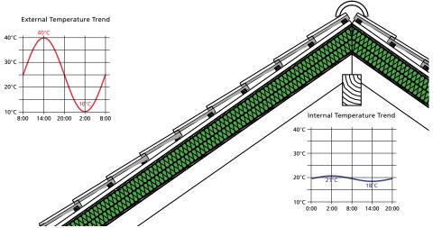
Amplitude Dampening and Phase shifting are as vital for summer heat protection as the U value is for Thermal insulation in winter. Amplitude Dampening shows the strength with which the temperature penetration is reduced. The Phase Shift shows, by how many hours, the penetration of the maximum temperature is delayed.
